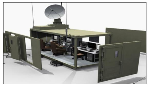
The CQT Weapon Systems Remotely Piloted Aircraft (RPA) cockpit housed in either a customer-furnished building or a mobile shelter and used to control one ISK-RS drone & give a comprehensive picture of the battlespace. Its is set up primarily for remote operations via a Satellite Communications (SATCOM) data link. Ground- based radios can also be used.
